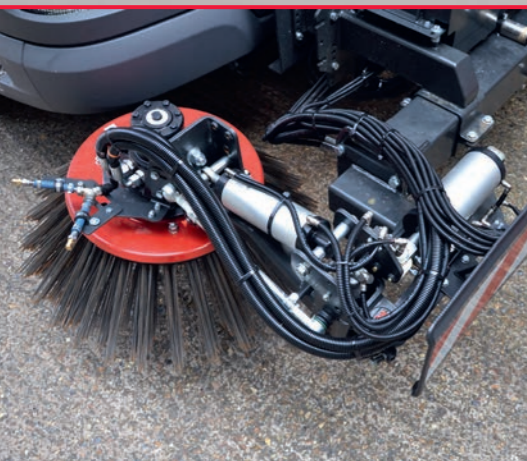
Front brush option 700 mm weedrip brush on a telescopic arm for long 1000 mm reach with in cab control.
