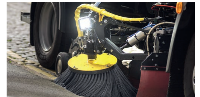
Triple sweepgear worklights LED worklights to illuminate the side of the sweeper and kerb.
