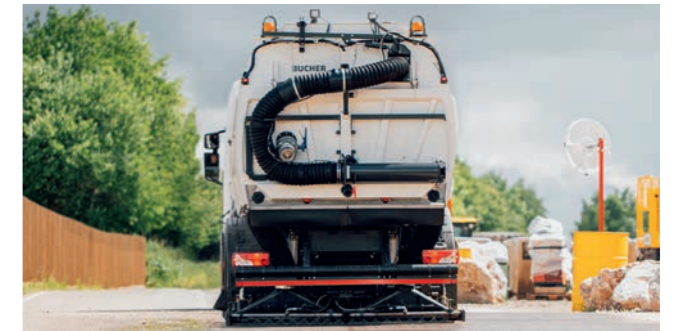
Rear mounted wanderhose Heavy duty 200 mm dia hydraulically powered wanderhose, mounted to the rear door, particularly useful for use in areas where there are height restrictions.
