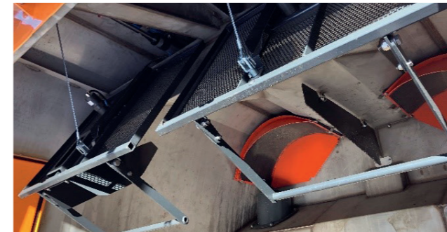
Remote mesh lift Allows the hopper meshes to be lowered and lifted into place remotely, without the need for the operator to stand in the dirty area.
