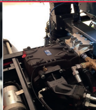
Powawash option High pressure water delivering 100 l/min @ 200 bar to a variety of spraybar options.
