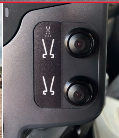
Rear nozzle operation Operation from the JVM with separate selection for low pressure water.
