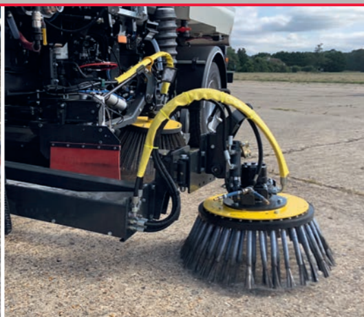
Side slide brush Optional brush behind the front wheel for increased swept width and effective weed removal without the use of chemicals.
