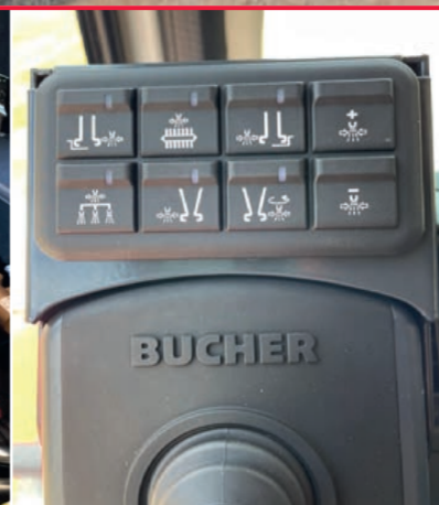
Powawash keypad Electronic water valves with in cab control for Powawash options.
