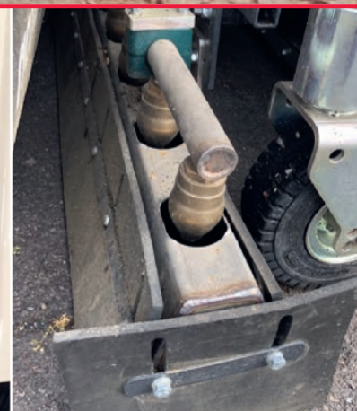
Rotating jets Optional rotating jets for high intensity cleaning in front of the rear nozzles.
