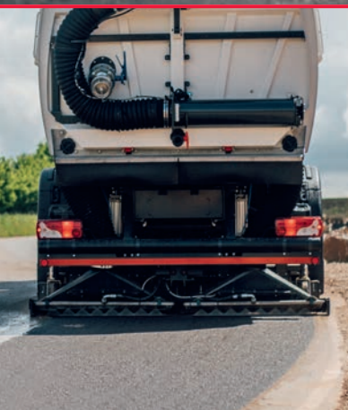
Rear suction nozzle option Full width nozzles for high performance pick up ideally suited for highways and road construction.
