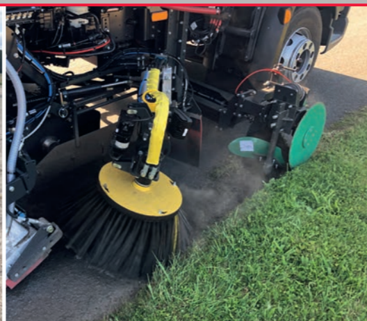
Disc coulter option Provides the ability to cut back turf ingress on non-kerbed roads and provides a neat clean cut edge to verges.
