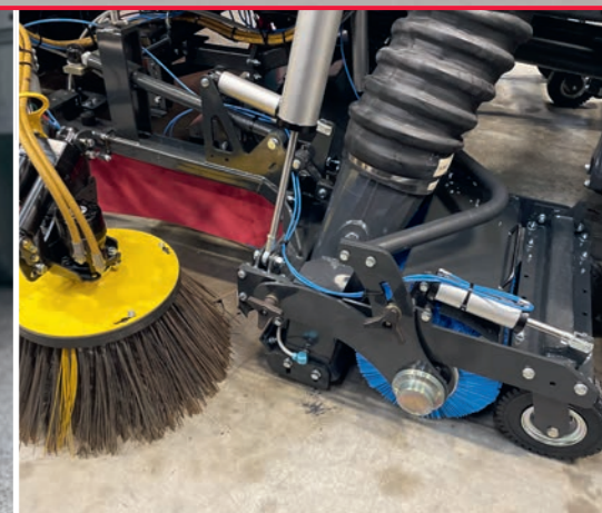
Broomvak sweepgear For high speed pick-up. Also allows pick up at reduced fan power in less demanding applications.
