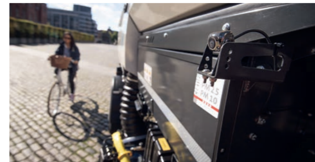
Quad camera Offside road view, providing additional vision for potential blind spots.
